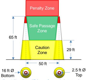
Figure 1: Dimensions and flight zones for a standard set gate pylons.
