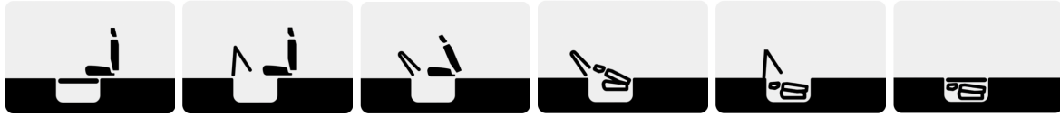
Figure 7.3 Stow 'n Go™ folding mechanism (from Ref. 102)
