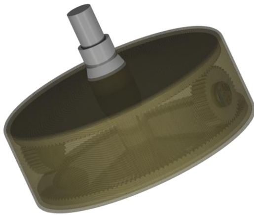
FIGURE H-2: ODYSSEY GEAR HOUSING IN GRAPHITE-EPOXY MATERIAL
