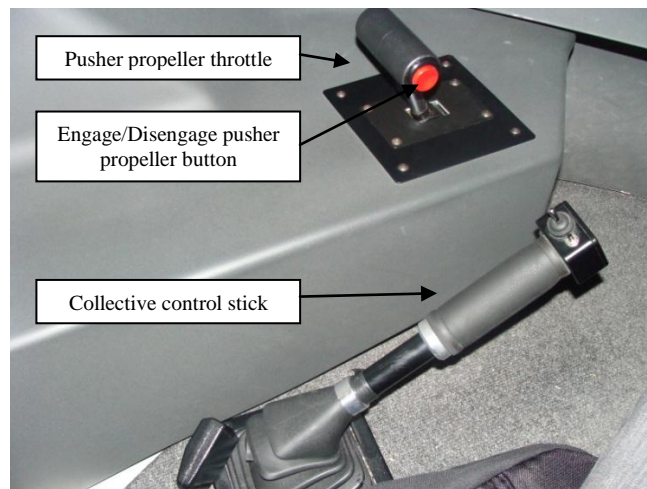
FIGURE M-15: ARRANGEMENT OF THROTTLE AND COLLECTIVE CONTROLS
