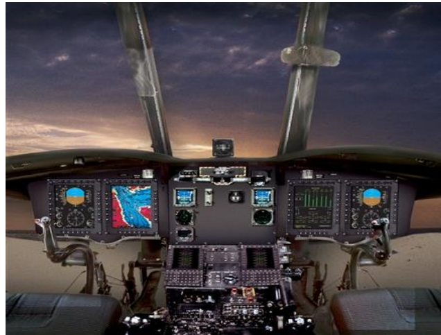
Figure 66: MH-47G cockpit mockup utilizing Rockwell Collins CAAS system 15
